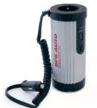
Salicru's **SPS AUTO** units are converters that supply the necessary electrical power in 230 VAC and 5 VDC. The input connection using the car (or ship) lighter socket and the 230 VAC schuko output has a power of 150 W, whereas the 5 VDC output is via USB port with a charge of 2 A.
